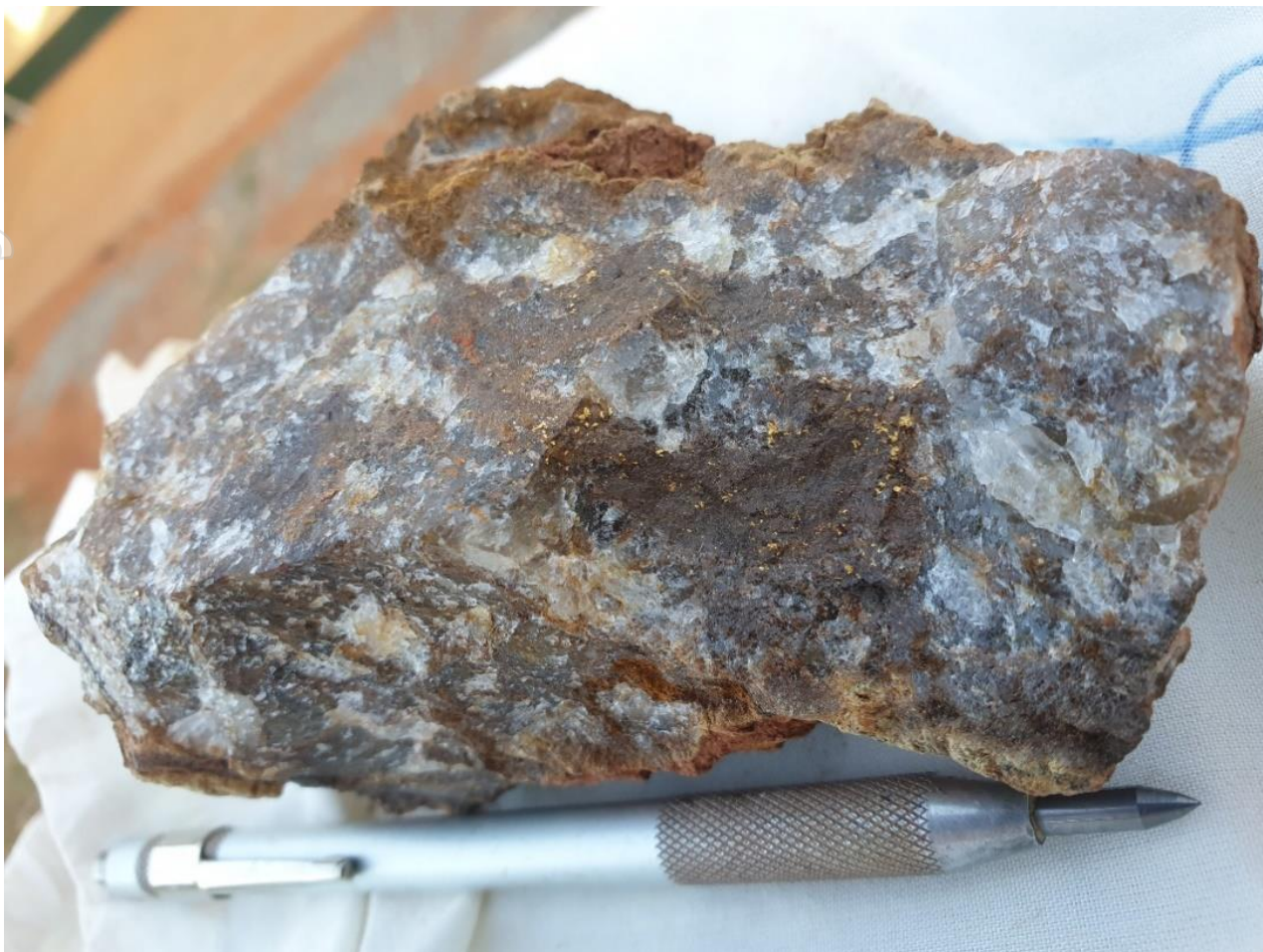
Figure 3: Photograph of a weathered, gossanous quartz vein with abundant visible gold recently sampled by Silver City from the outcrop exposures in the north face of the Brians historic pit.
