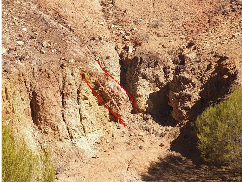
Figure 5: Photograph looking northwest into the historic Buccaneer showing the gossanous fault zone with associated quartz veins (red dash outline) trending northwest and dipping northeast.
